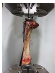
Fig.2-2 Mounted specimen on the Fatigue tester
